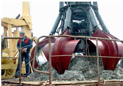
Hydraulic grab with TV-control (for hard rock)
